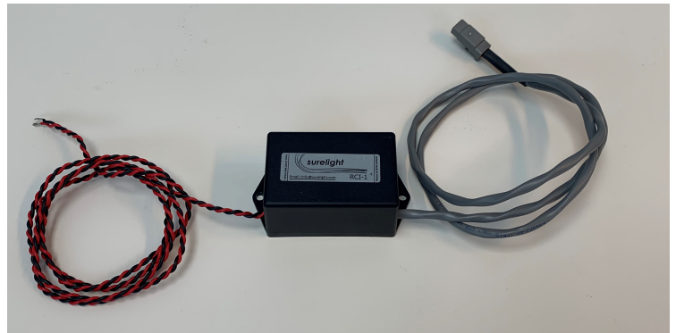
Twisted cables used on both low voltage DC input and high Voltage AC output of RCI-1 inverter. Fuel resistant heat shrink applied to output cable and heat shrink boot fitted to female 2 pin Deutsch connector, which mates with corresponding male Deutsch on EL panel.
